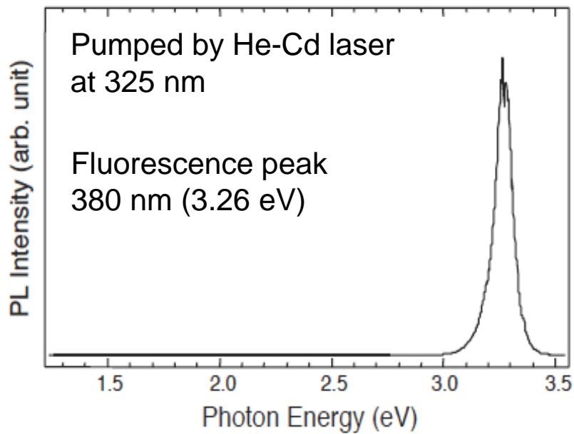
ZnO Crystal grown by hydrothermal method
