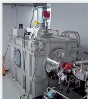
A high-quality electron beam is launched from a CeB<sub>6</sub> electron gun.
