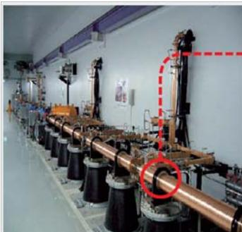
The C-band accelerator swiftly increases the electron energy.
