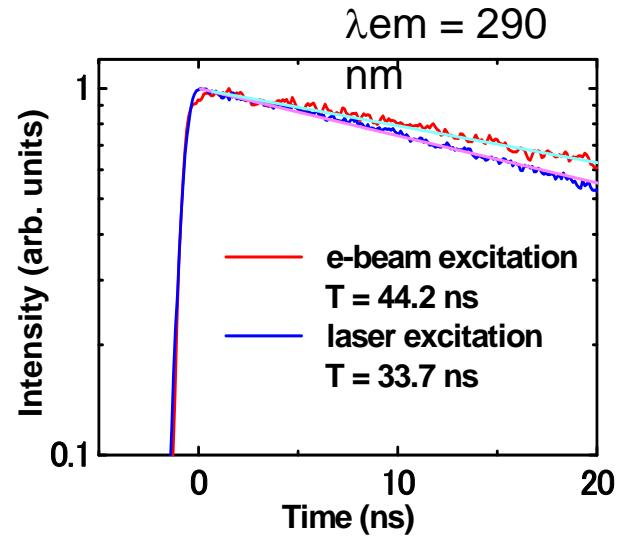
In the case of e-beam excitation of Ce:LiCAF, fluorescence lifetime became longer
