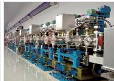
The in-vacuum undulator generates strong XFEL radiation.
