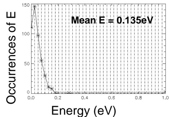
Ar: dominated by low-T “thermal” background – improved sampling needed to capture high-energy tail.
