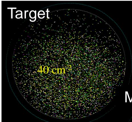
Shadow of wafer in front: defects arrive line-of-sight from gun/target area
