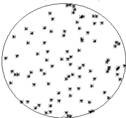
Model did not have "shadowing" wafer in front: no shadowing expected. Gravity bias reproduced by model.
