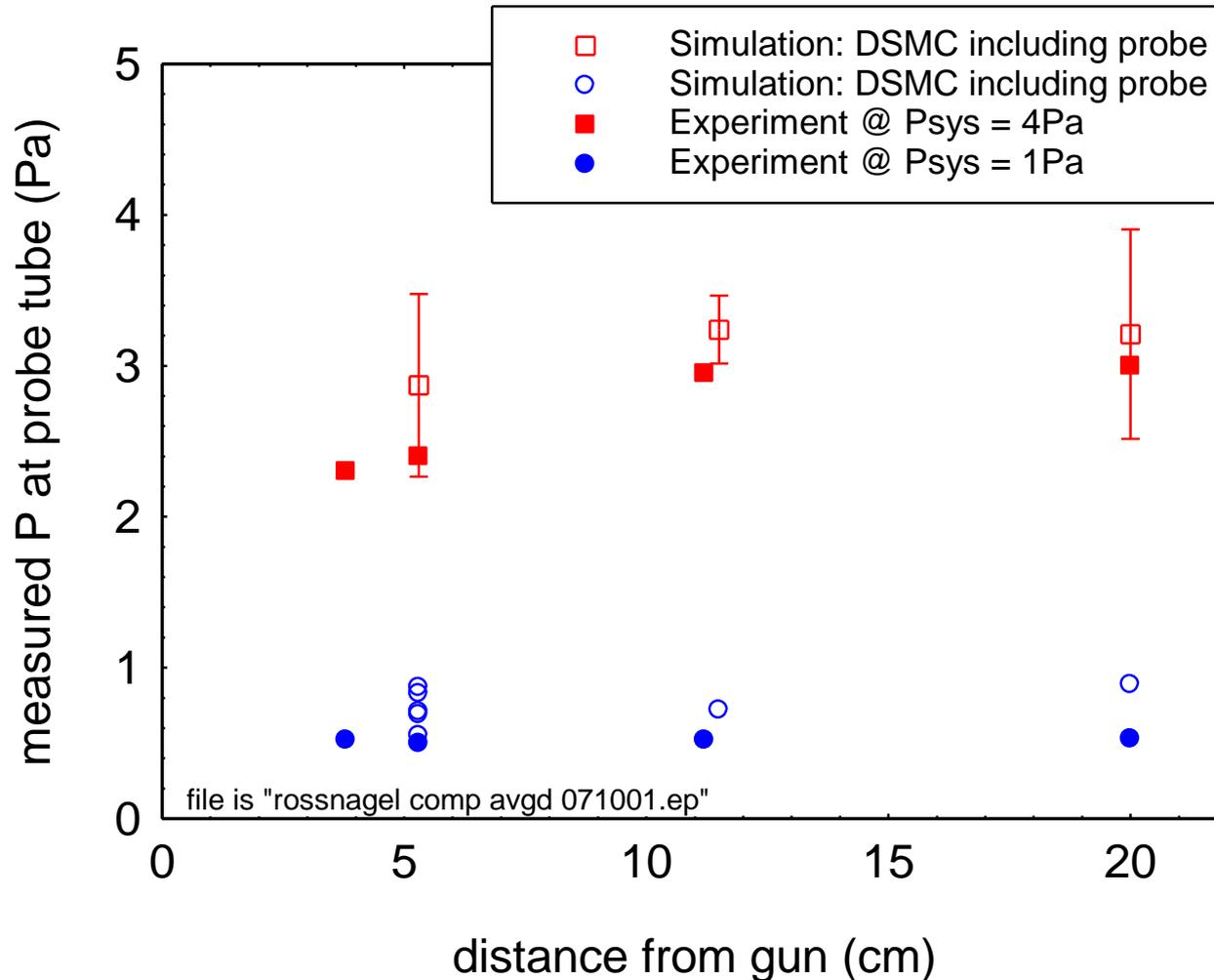
Scatter in simulation results comes from instability in simulated pressure inside the measurement tube – working on whether this is an artifact of radial weighting.
