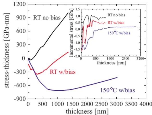
Experimental results: becomes more tensile with thickness under a variety of conditions.
