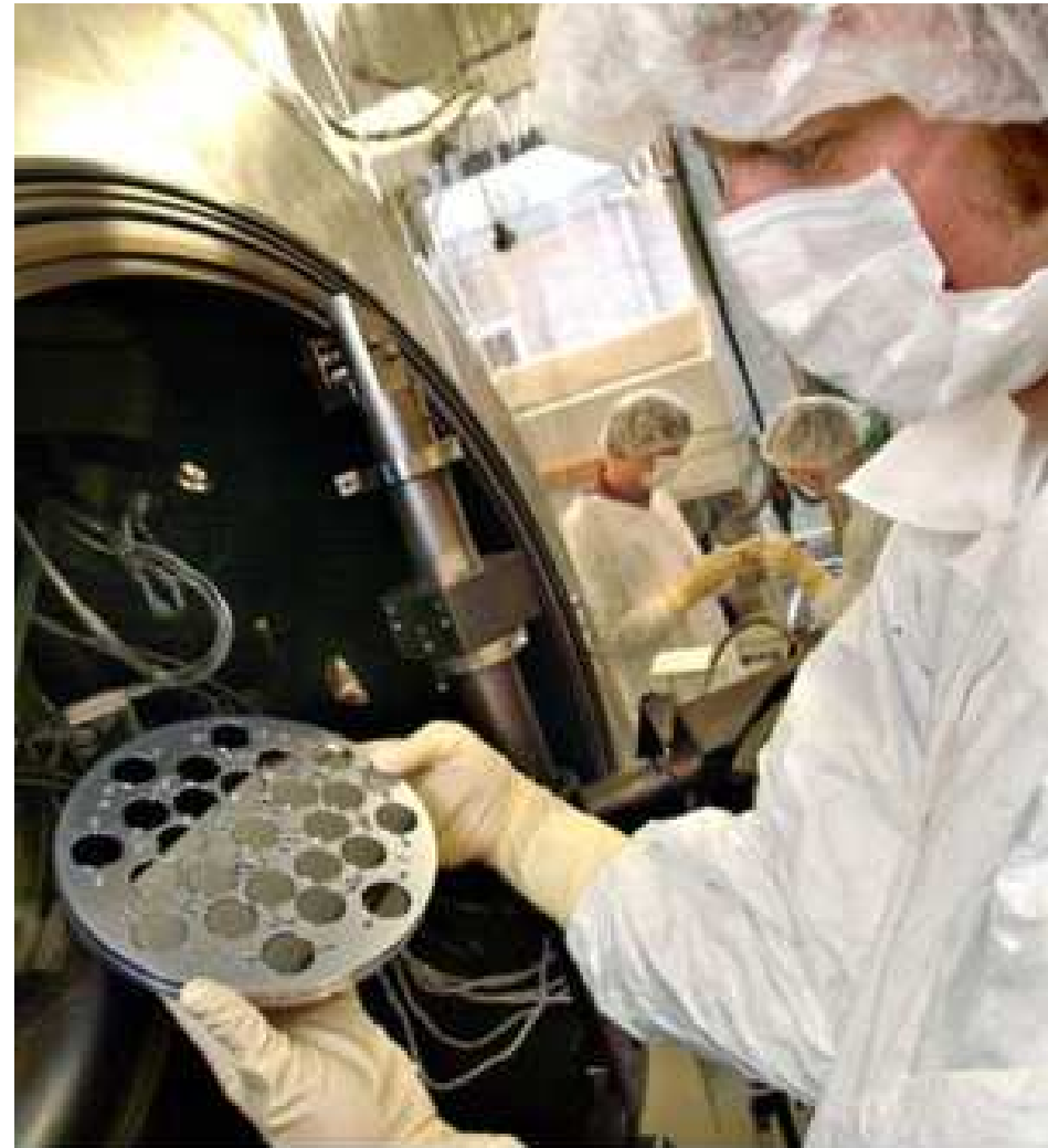
Demounting of a batch of multilayer test samples in one of the nSI UHV deposition systems (photo by N. Steenkamp)
