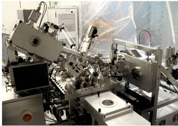
EUV Technology Outgassing Tool Installed at IMEC
