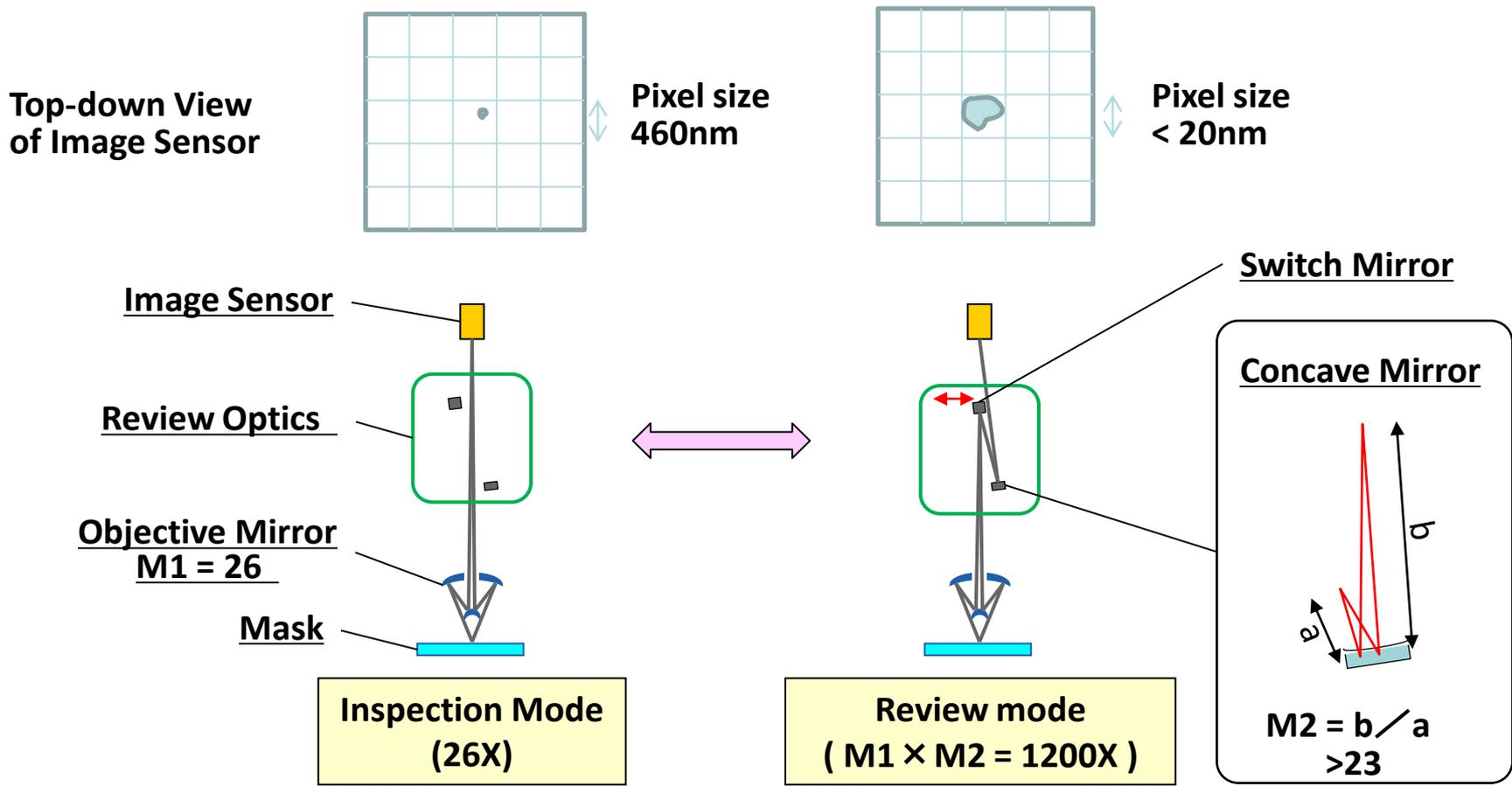
✓ Review optics enables to demagnify the corresponding pixel size of image sensor on wafer and to identify the position of phase defect with higher accuracy.
