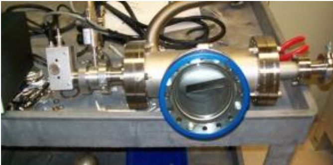
Test chamber at CXRO used for cleaning Si-capped EUV optics
