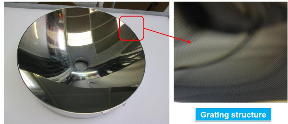
Demonstration Collector: ~450mm dia (NA ~0.23)
