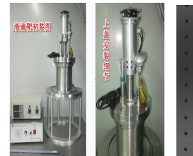
Photograph of droplet generator and the generated water droplets
