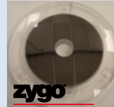
EUV ML Coated M1 and M2 mirrors
