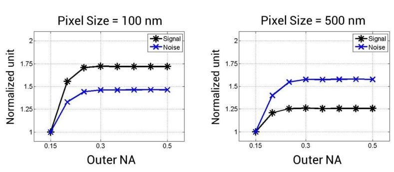
Increasing photon collection efficiency by larger outer NA doesn't necessarily increase defect SNR. It is pixel size dependent and the impact saturates at NA > 0.3.
