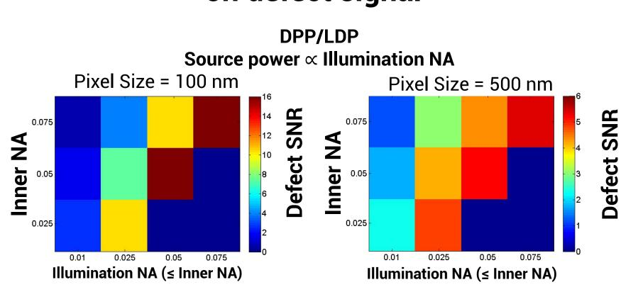
Illumination NA = Inner NA has max. defect SNR. Larger partial coherent illumination (more photons) is better.
