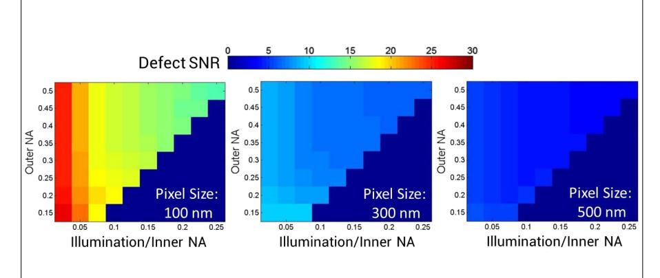
Pixel size is the dominant factor on defect SNR compare to NA of the optics under fixed photon density.
