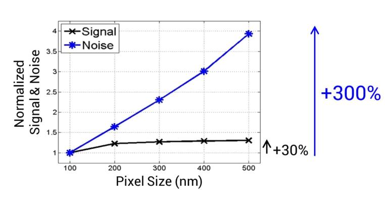
Larger pixel size reduces the inspection time but also increases the noise more than the defect signal.
