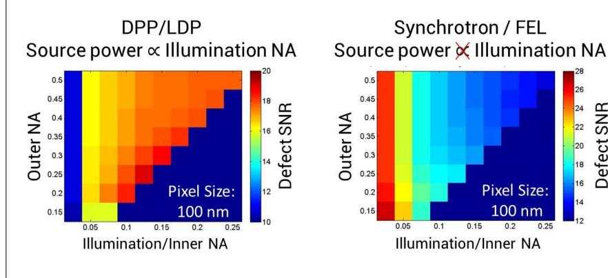
At signal shot noise dominated situation (pixel size = 100) nm), larger illumination NA (partial coherence) improves the defect SNR by more photons for DPP/LDP source.
