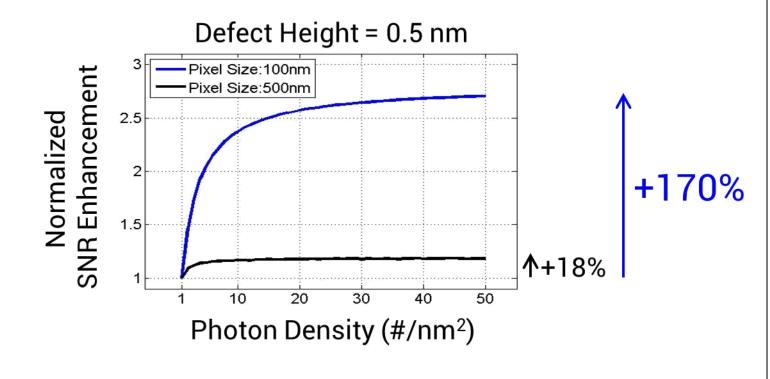
SNR enhancement by increasing source power saturates faster and the enhancement is smaller at larger pixel size.
