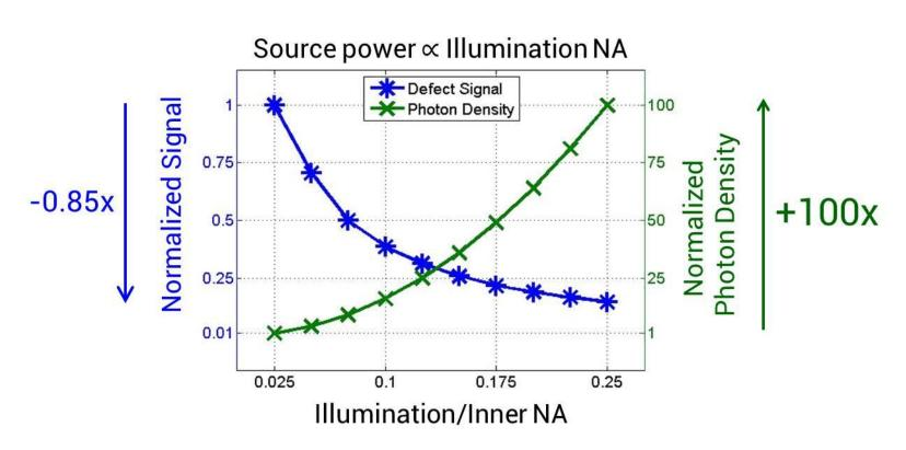
Increased source power compensates the loss by larger partial coherence and increases the signal strength in abs. number of photons.
