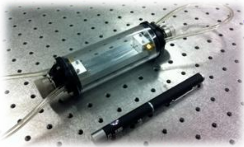
High pressure waveguide Excellent coherent buildup and flux
