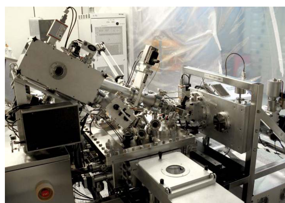
LithoTech outgassing tool at Selete [7]
