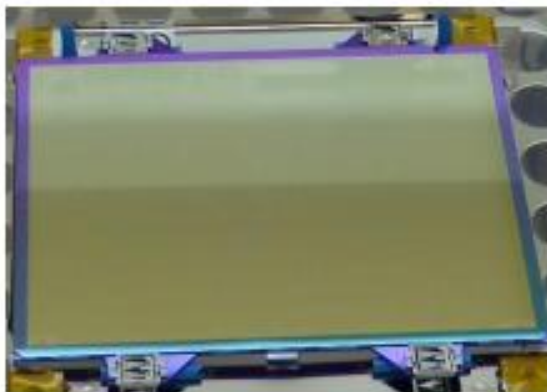
Pellicle Film EUV Transmission
