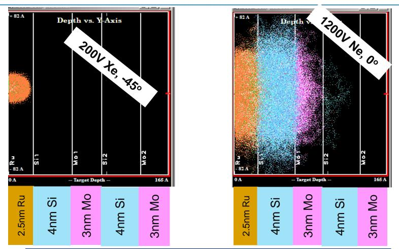
Ion damage can be limited by appropriate combination of ion species, ion energy and fixture angle
