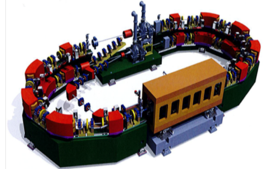
Cosami: Mini synchrotron for EUV High brightness Small footprint: 5 \times 12 m 2
