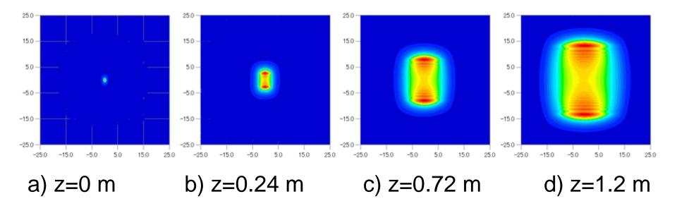
Divergence of FEL light due to diffraction effect between the undulators. z is the distance from the 1st undulator.
