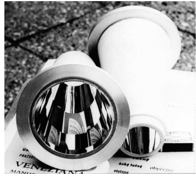
Electroformed X-ray mirrors (hyperbolas, Ni surfaces, Acad of Sci, Prague)
