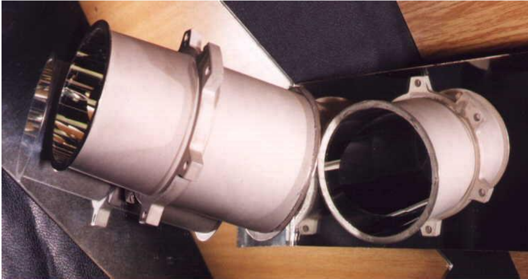
Electroformed Wolter X-ray Mirrors for Space Research (aperture 80 mm)
