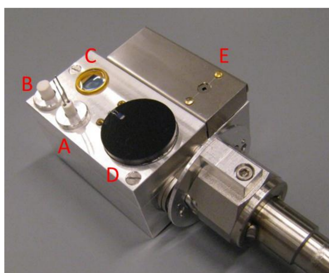
Figure 1: Sensor head with Langmuir probe (a), PT100 (b), photo diode (c), heat flux sensor (d) and Faraday cup (e).
