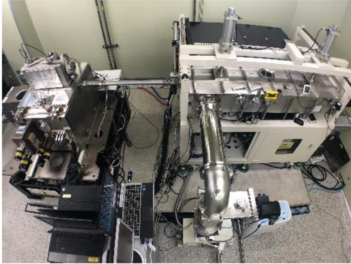
① Capture the diffraction patterns using EUV-ptychography microscope
