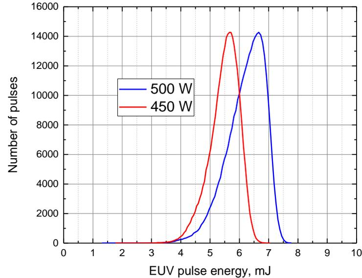
*Open loop, 15 ms Bursts, 80 kHz,
