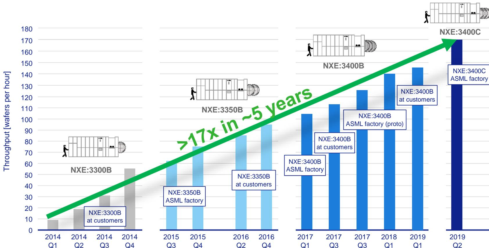
ATP test: 26x33mm<sup>2</sup>, 96 fields, 20mJ/cm<sup>2</sup>
