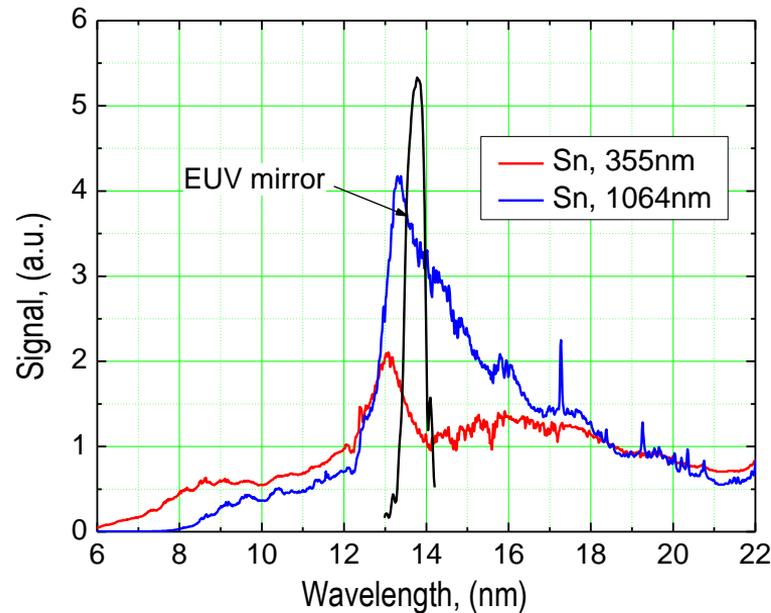
Peak of EUV spectrum matches the MoSi multilayer reflectivity band at 13.5 nm
