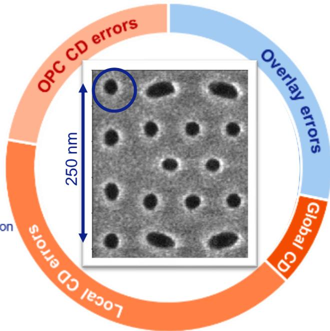
Edge placement error (EPE): combined error of overlay and CD uniformity (global CDU, local stochastic and OPC error)
