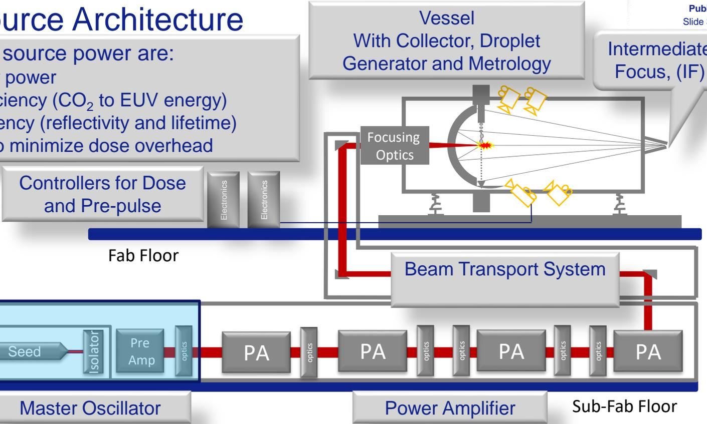
$$\text{EUV power (source/scanner interface, [W])} \propto \text{CO}_2 \text{ power [W]} * \text{Conversion Efficiency} * \text{1 - Dose Overhead}$$
