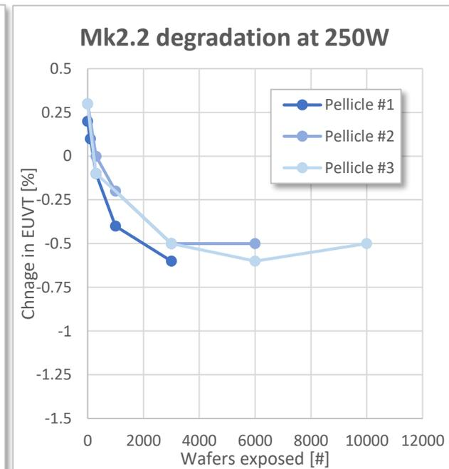
*NXE:3400B @ 250W, 96 fields per wafer, 50mJ/cm<sup>2</sup> sensor based, 35mJ/cm<sup>2</sup> in resist
