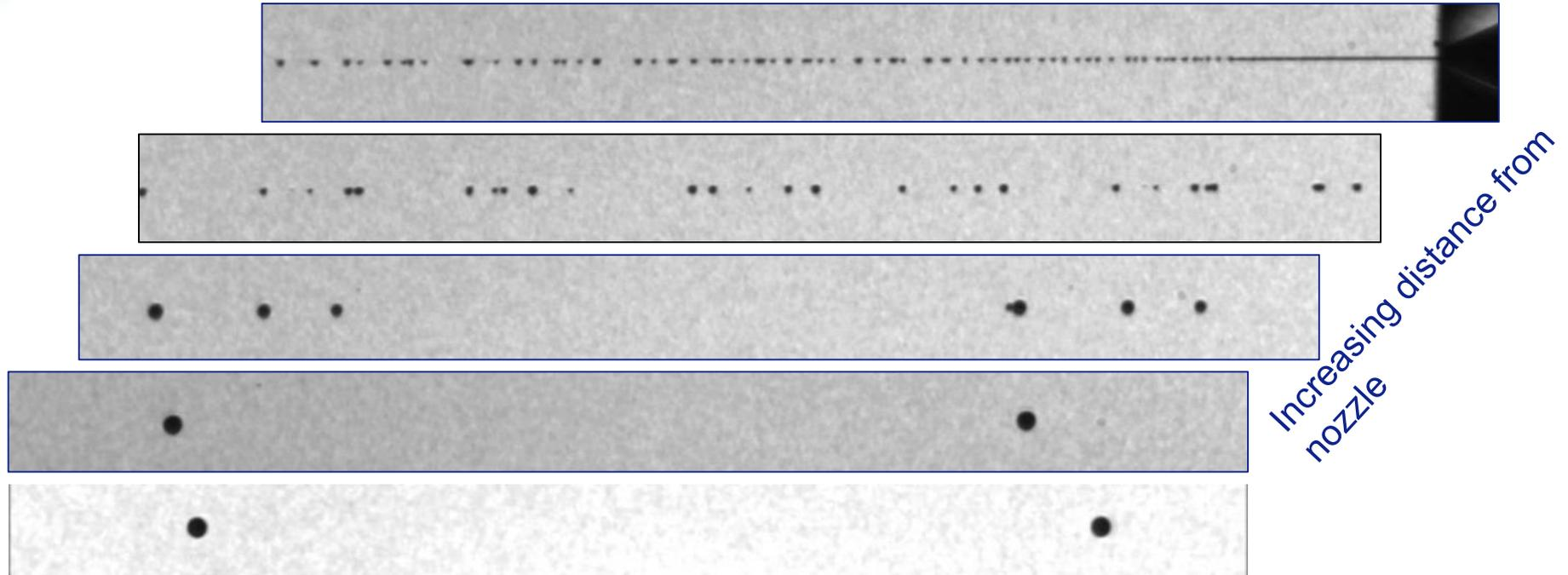
Multiple small droplets coalesce together to form larger droplets at larger separation distance
