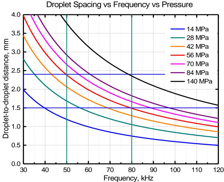
Droplet spacing of 1.5 mm demonstrated at 80 kHz
