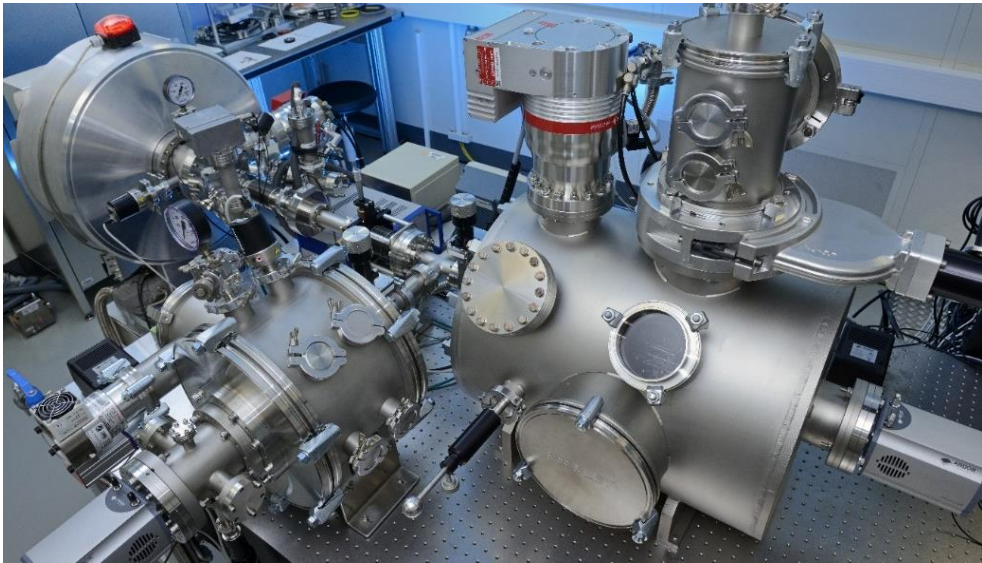
EUV Dual Beamline in research configuration (footprint: 2.5 x 1.5 m 2 )
