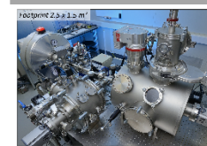
UVI dual beamline for nanopatterning at 10.9 nm and 13.5 nm.
