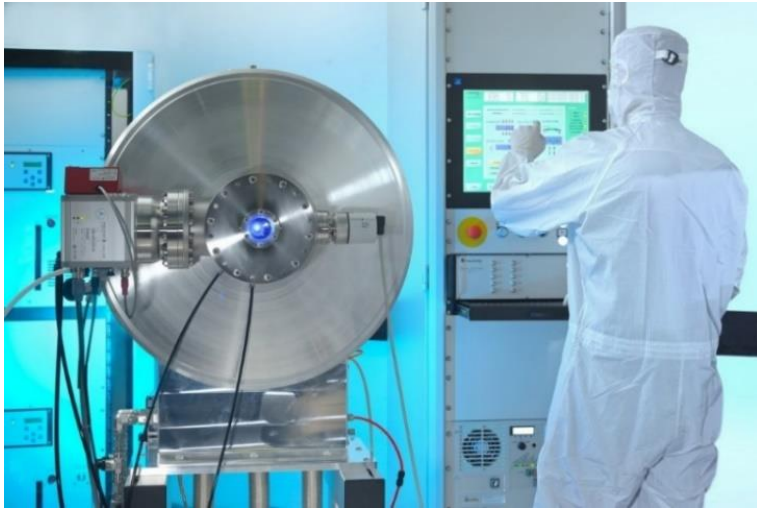
Commercial EUV source (FS5440, Fraunhofer ILT)
